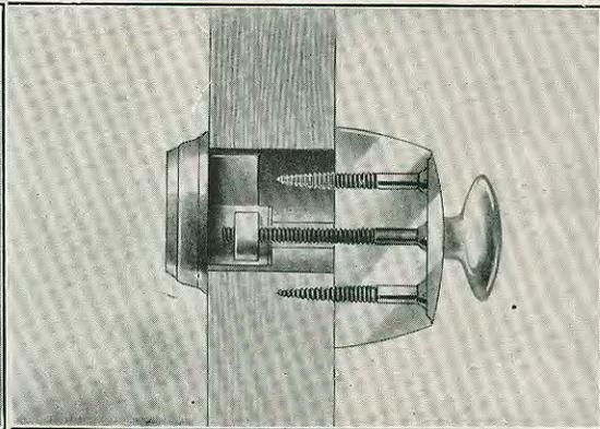
Illustration shows lock case and cylinder held in place with one hand while connecting screws are applied with the other. The simplest and quickest method in use in applying a dead lock or a night latch. The Nos. 341 and 326 Night Latches, and No. 330 Dead Lock can be applied to doors in one-half the time required for other cylinder locks.
